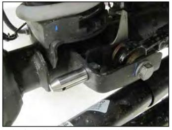
O Attach the long mounting post with polyurethane spacer into the factory sway bar link mount. The stud should point towards the center of the vehicle. Tighten the post ensuring the click pin hole is horizontal or parallel with the ground. Tighten to 65 ft-lbs.
