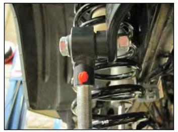
Measure back 1-1/4" from the center of the sway bar link hole or just past the weld at the axle and make a vertical cut line. Cut off the tab at the mark and paint exposed metal.
